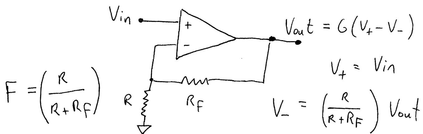
$V_-$  = potential between  $V_-$  and ground, which is the same as  $V_R$ .
