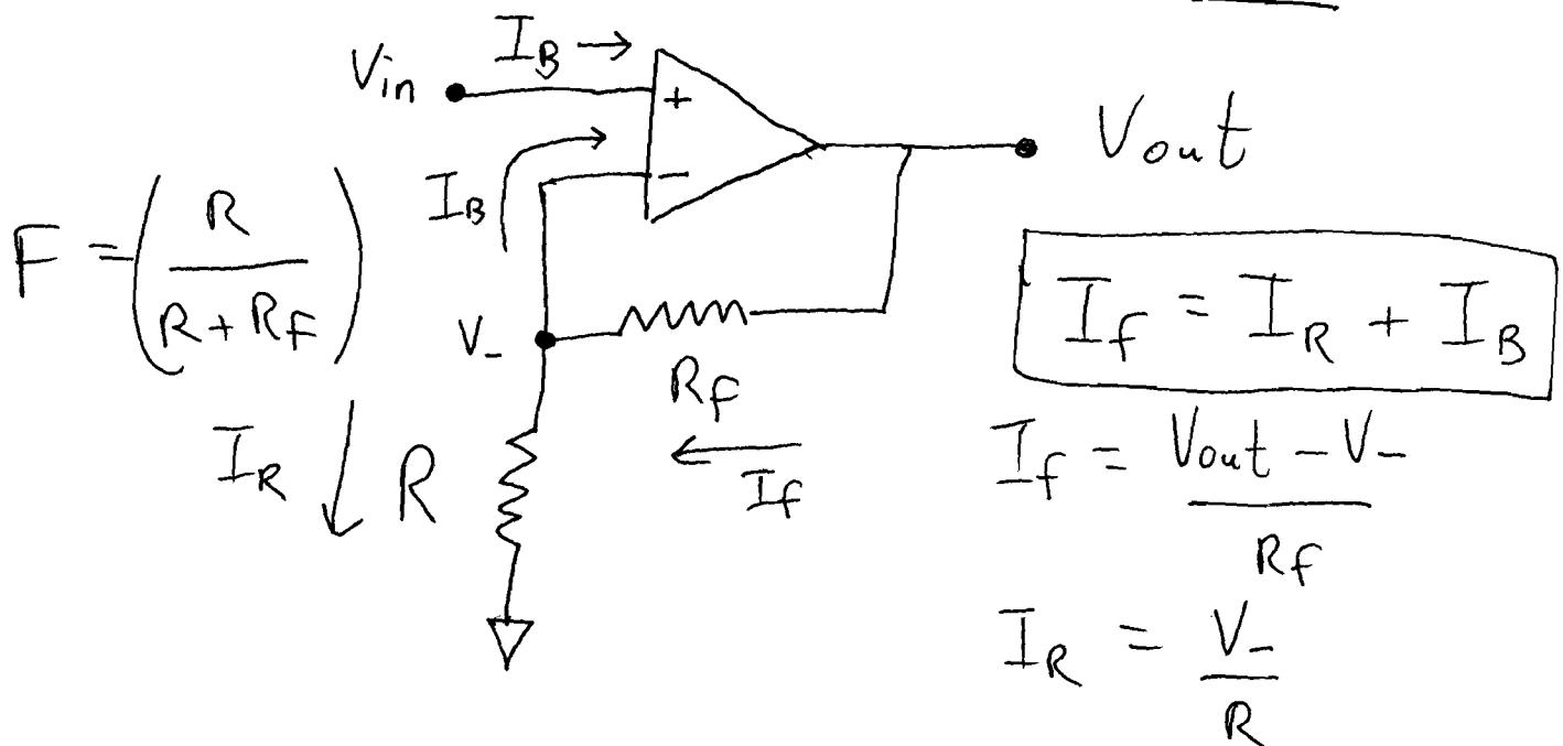
$$I_f = I_R + I_B \text{ implies } \frac{V_{out} - V_-}{R_F} = \frac{V_-}{R} + I_B$$
