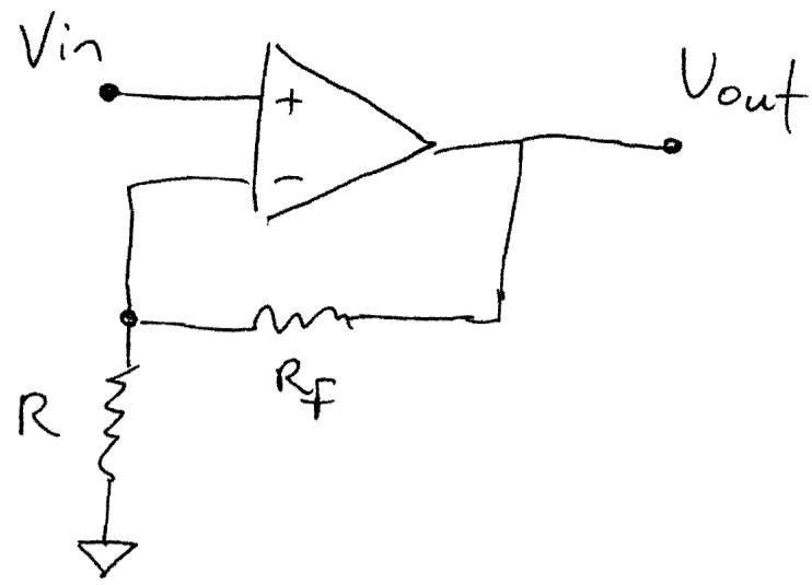
$$V_{\text{out}} \approx \frac{1}{F} V_{\text{in}} = \left( \frac{R + R_f}{R} \right) V_{\text{in}}$$
